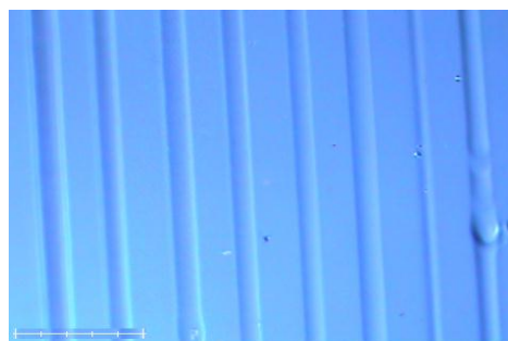
Figure 3. Lines written in a lead vanadate glass (785 nm, 40 mW)
